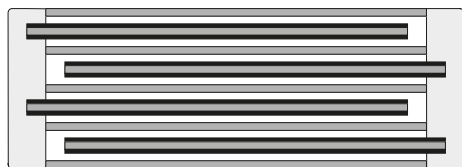
Extended double side metallized carrier film design
