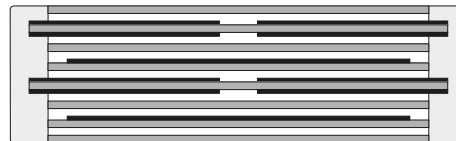
Extended double side metallized carrier film design with internal series connection and metallized film (series connection of 2 elements)
