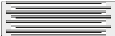
Extended metallized film design
